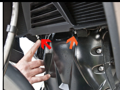
4 Loosen two T25 Torx screws securing the front cover & radiator 3-4 turns. DO NOT REMOVE.
